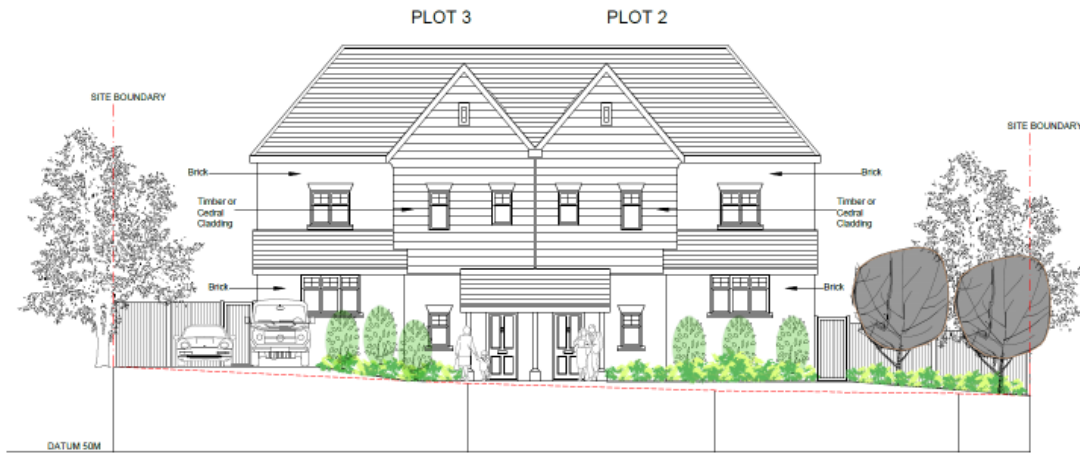
Front Elevation (West)
